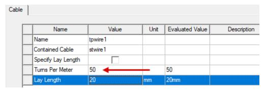
Notice that the *Lay Length* (that is, the distance for one full 360-degree twist) is updated automatically to 20 mm.
